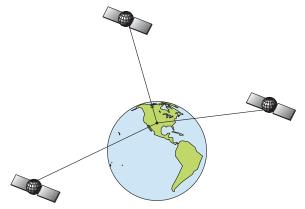
Three satellites are required to determine a 2D fix.
